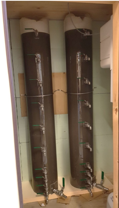
Fresh tunnel wash water in the sedimentation pilot
