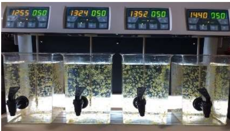
Example of jar test after pH adjustment and dosage of polymer
