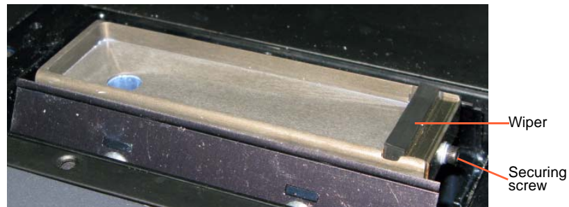
Figure 7-30: Wiper and excess-material drain
