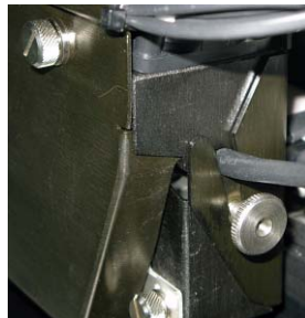
Figure 7-74: UV-lamp cable after replacing the assembly
