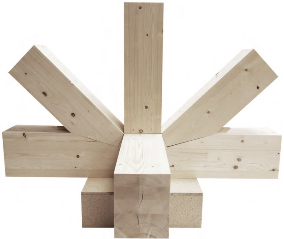
Detail 1 built in scale 1:1, improved version of compression joint
