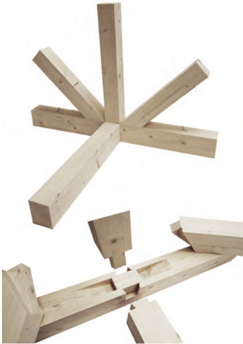
Detail 1 built in scale 1:2, testing the joint with most compression
