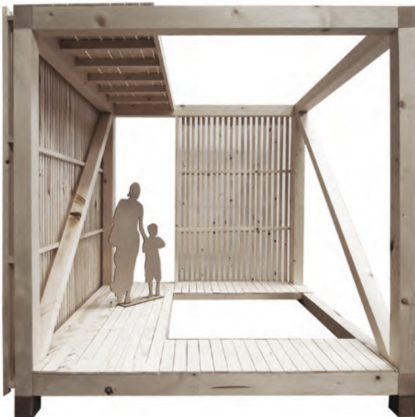
Model in scale 1:5 of the fireplace box
