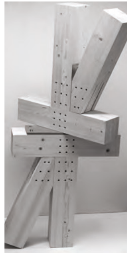
connection point scale model 1.1
