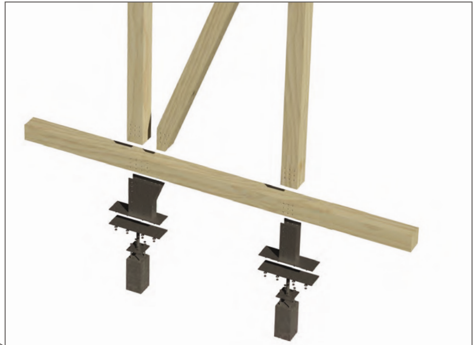
base point explosion drawing
