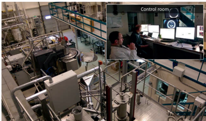
Figure 2: The silicon production laboratory at IFE. Inset: The control room from which all pilot reactors are controlled remotely to ensure the safety of the operators.
