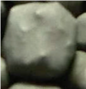
Figure 12: The particle shown is around 2.5 mm in size. Scavenged particles appear as bumps on its surface.
