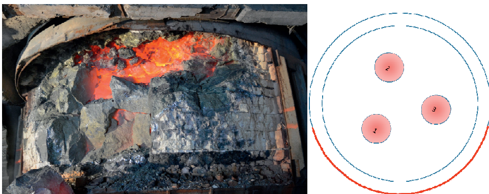
Figure 6: Pictures of furnace no.1 in Wacker with marked excavation front.
