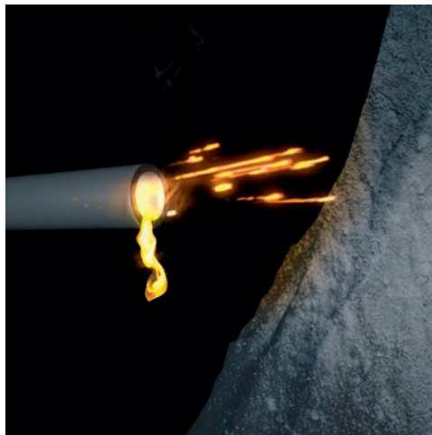
Figure 2. Remaining sparks when standard lance is removed from surface
