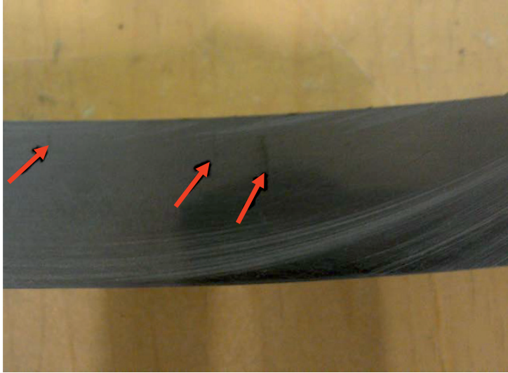
Figure 3: Wall cross section, showing the crack depth and morphology.
