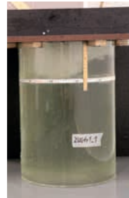
Figures WP2_3 Test set-up for the ice rubble packing experiments: 1 – packing table, 2 – guiding plank, 3 – plexiglass cylinder filled with saline water, 4 – ice rubble & Figure WP2_4 An example of ice rubble packing test performed in the cold laboratory at NTNU
