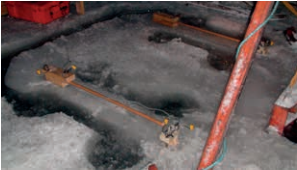
Figure WP1_4. In-situ test for tensile strength of floating ice
