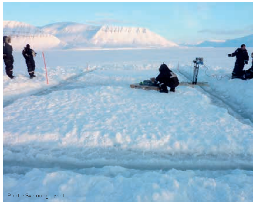
Figure WP4_4. A trial campaign in the field to acquire the fracture properties of sea ice.
