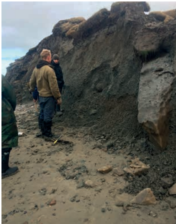
Figure WP6_4 Sampling from different parts of the coastal sediments at Baydaratskaya Bay for later laboratory work.
