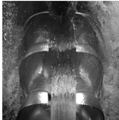
Flow in a bucket. This picture is taken with 25 m head, nozzle opening of 10 mm and n_{11} = 38,5 .
