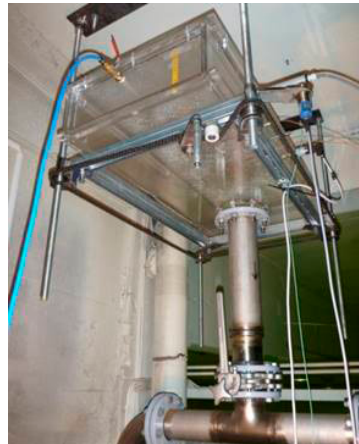
The air cushion surge chamber in the physical model
