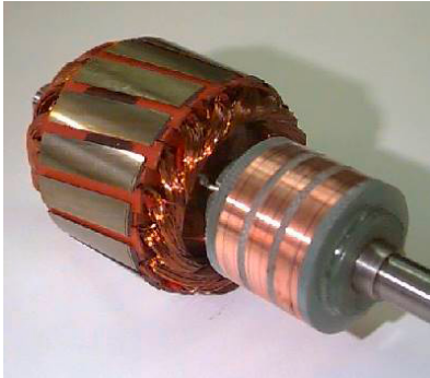
The wound rotors used in the motors at the pump station are likely to play a part in creating the disturbance.
