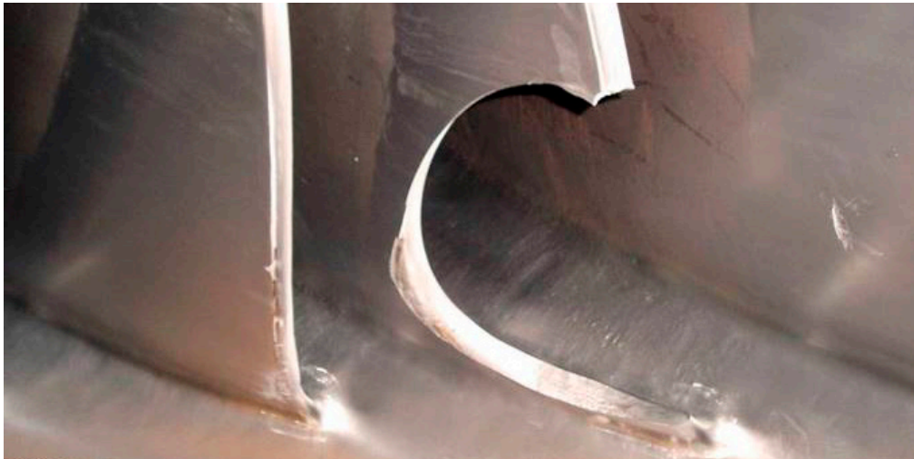
Damaged runner, Svartisen, Norway
