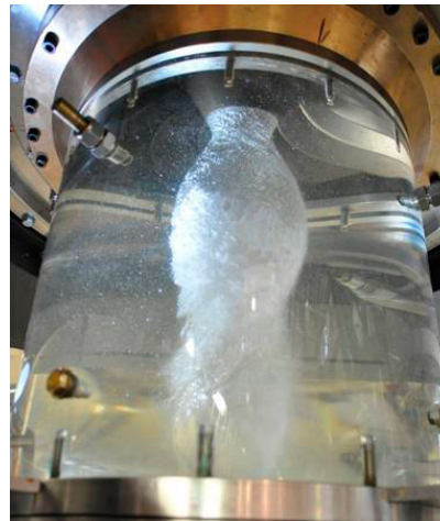
Frequency analysis of a pressure pulsations in a Francis draft tube
