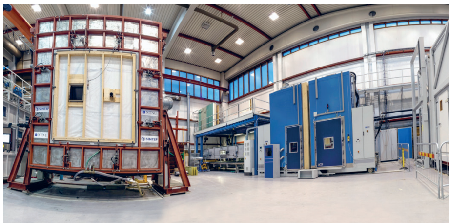
Figure 1. The figure shows a panorama view of building physics laboratory with rotatable hot box (grey box to the right), climate simulator (blue box in the middle), and RAWI box (rain and wind box, to the left). Photo: SINTEF Building and Infrastructure.
