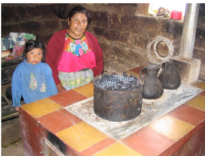
Figure 2. The Plancha chimney stove, Guatemala (photo Anaite Díaz).
