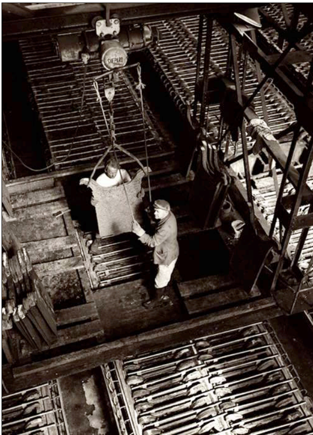
Nickel electrolysis, changing of anodes, Falconbridge Nickel Refinery (Kristiansand), 1960. Unknown photographer.
