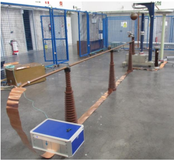
Fig. 11 – Magnetic field testing set-up.
