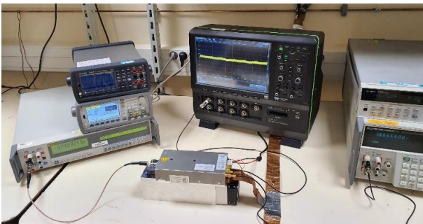
Fig. 5 - Testing amplifier D at DC/AC voltages
