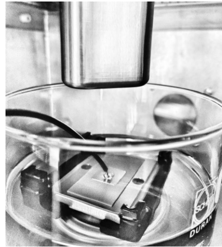
Fig. 13 – Liquid light guides positioned above the ceramic substrate in silicone liquid to detect visible PDs. The HV electrode is on the bottom of the sample holder.
