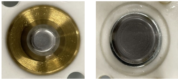
Fig. 7. Left: conical top electrode (d=12 mm), Right: cylindrical top electrode (d=25mm). In both cases the bottom electrode is a cylindrical electrode (d=25mm)
