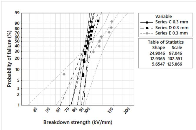
**Figure 5.** Breakdown strength on 0.3 mm test objects using semi-spherical electrodes in oil 2 with (Series D and E) and without (Series C) silicone embedded electrodes.
