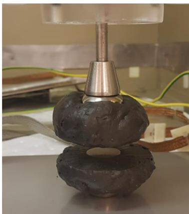
**Figure 2.** Spherical electrode system molded with silicone rubber.
