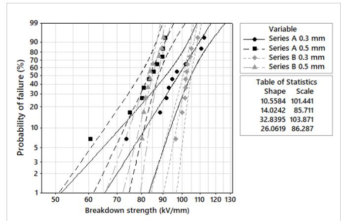
Figure 3. Comparison of breakdown strength between oil 1 (Series A) and oil 2 (Series B) using IEC electrodes.
