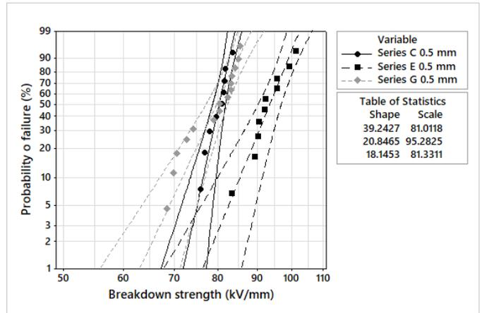
**Figure 8.** Breakdown strength on 0.5 mm test objects using semi-spherical electrodes in oil 1 and oil 2 with and without silicone 2, where the combination of oil 2 and silicone 2 (Series E) has a combined effect on the breakdown strength compared oil 1 and silicone 2 (Series G).
