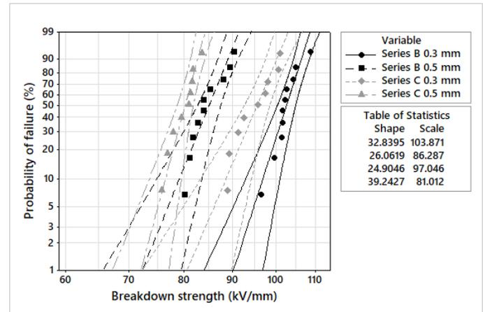
Figure 4. Comparison of breakdown strength between IEC (Series B) and semi spherical electrodes (Series C) performed in oil 2.
