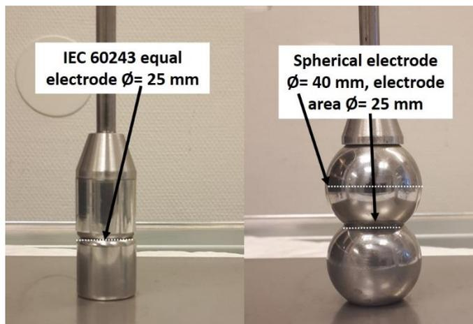
**Figure 1.** Electrode system according to IEC 60243 to left and partially-spherical electrodes to right.
