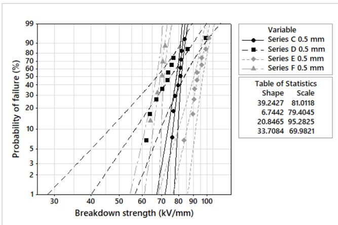
**Figure 6.** Breakdown strength on 0.5 mm test objects using semi-spherical electrodes in oil 2 with (Series D, E, and F) and without (Series C) silicone embedded electrodes.
