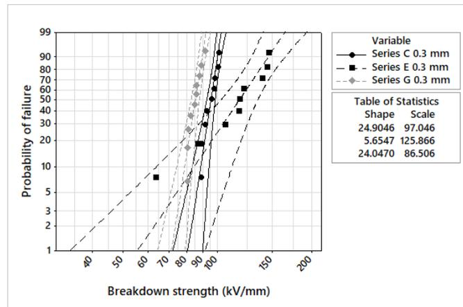
**Figure 7.** Breakdown strength on 0.3 mm test objects using semi-spherical electrodes in oil 1 and 2 with and without silicone 2, where the combination of oil 2 and silicone 2 (Series E) has combined effect on the breakdown strength compared oil 1 and silicone 2 (Series G).
