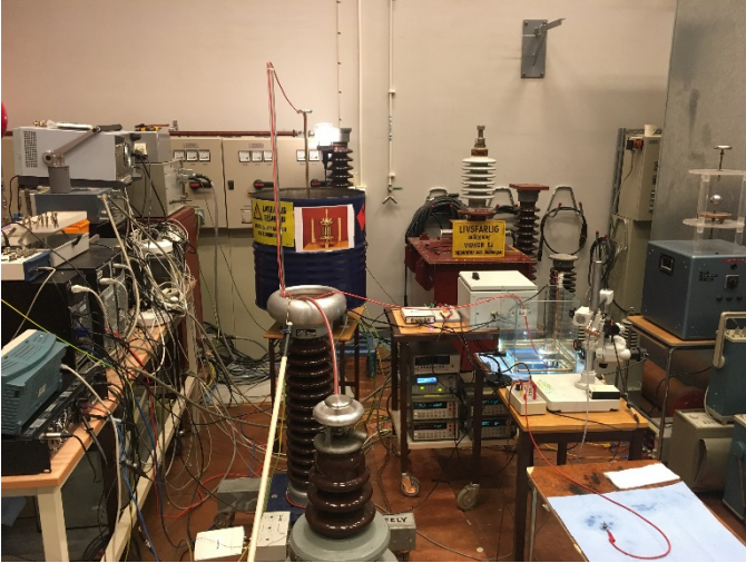
Figure 4. The setup which facilitates the electrical tree inception experiments.
