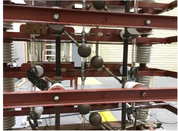
Fig. 9 – Components within a single stage of the MSU impulse generator.
