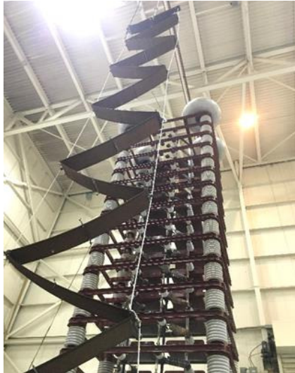
Fig. 12 – zigzag design of external tail resistors R_2 .
