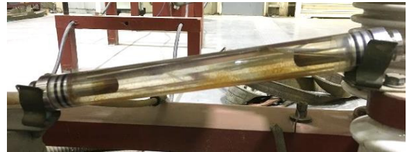
Fig. 10 – Charging process changes water properties within resistors over time as evident from the discoloration.
