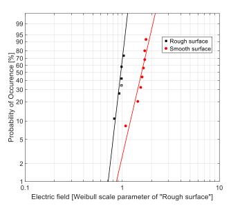
Figure 8 Weibull plot of breakdown measurement results normalized by Weibull scale parameter ( $\alpha$ ) of curve "Rough surface".
