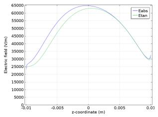
Figure 6 Simulated electric field in rubber-epoxy interface at applied voltage 1 kV peak. Absolute field (Eabs) and tangential field (Etan).
