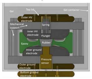
Figure 1 Schematic picture of test cell. During testing the gel container was partly immersed in insulating oil to prevent flashover.
