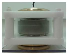
Figure 3 Photo of mounted inner part of test cell prior to gel filling.
