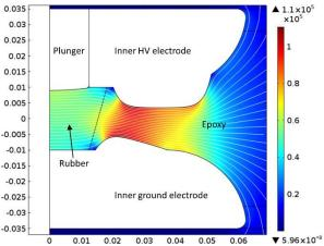
Figure 5 Simulated electric field distribution (color) and equipotential lines in inner part of test cell. Applied voltage 1 kV peak. Plunger extending 1 mm into rubber plug.
