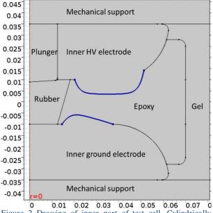
Figure 2 Drawing of inner part of test cell. Cylindrically symmetric around r = 0. Measures in meter. Protruding Rogowski-shaped parts of electrodes marked in blue.
