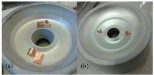
Figure 7 Shaped epoxy body painted with conductive silver paint (a) top surface, (b) bottom surface. Contacting strips of copper foil placed in silver paint to secure contact to metal inner electrodes.
