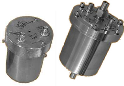
Fig. 1 – Test cells used. LHS CL-1 and RHS CL-2. For CL-2 has connections for hoses to measure flowing oil.
