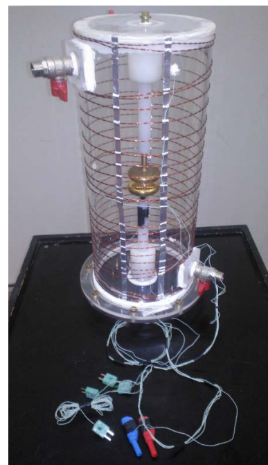
Fig. 2: Temperature and moisture controlled chamber, housing test object and electrodes. Clearly can be seen the heating wires wrapped around the chamber and the inlet and outlet for the cold gas.
