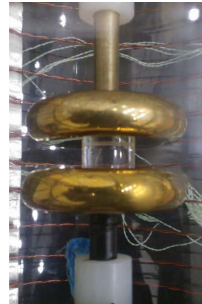
Fig. 1: PMMA test object between the plane parallel electrodes.
