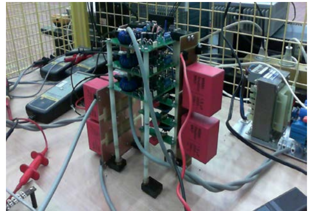
Figure 3. Buck converter set-up with three IGBTs in series in the laboratory. Compact structure leads to have low inductive circuit.
