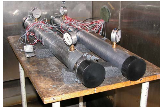
Fig. 3 – The two test objects with manometers attached, inside the heat cabinet. The sample with steel tapes is seen to the left, and the one without to the right.
