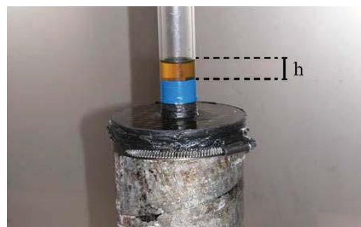
Fig. 1 - Test object for measuring impregnation level and cavity-free temperature. The height of the oil column was measured as a function of temperature, and the objects were kept around 24 hours at each temperature.
