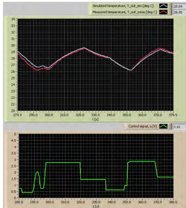
Figure 4: Result of adaptation of time-constant with time-delay model to the real air heater. Lower plot: Control (input) signal to the electrical heater. Upper plots: Real (measured) outlet temperature (red curve) and simulated outlet temperature (blue curve).
