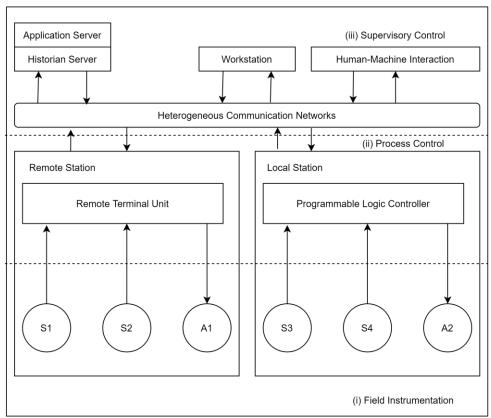
Figure 1: Typical Industrial Control System (ICS) Architecture
