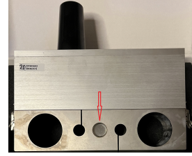
Fig. 4. The ICEBOX Line Sensor strain gauge.
