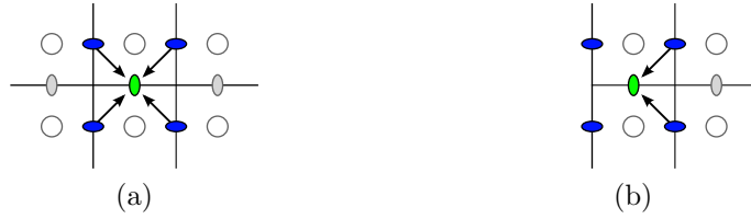
Figure 2: Reconstruction of physical quantities at other grid locations. The reconstruction of the horizontal velocity hu at (i + \frac{1}{2}, j) internal nodes (a) and boundary nodes for closed boundaries (b). The reconstruction of hu is similar.
