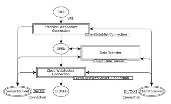
Figure 1: Client module of the WS CPN model.
