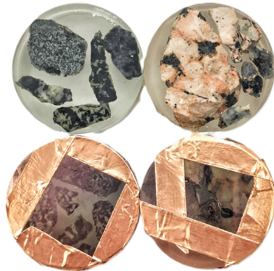
Photo of polished aggregate samples before and after SEM preparation.
