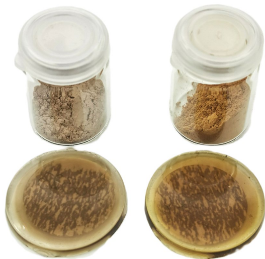
Photo of preheated powder and glass sample used for XRF.
