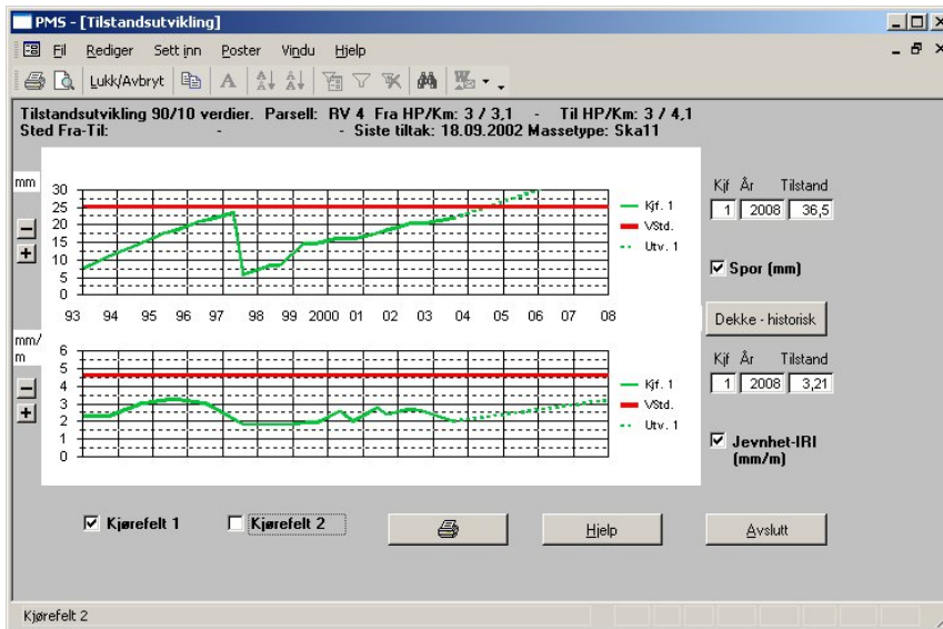
FIGURE 3: The historical and predicted development of rutting (top) and roughness (bottom) for a specific road section over the period 1993 - 2008. The red lines are target values.
