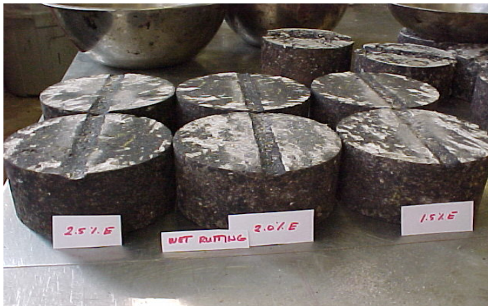
Figure 6: Laboratory Processed Cylindrical Samples After Rut Test in the APA [Salina Site]
