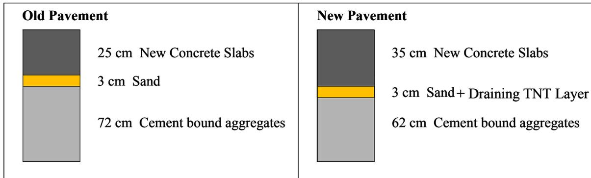
Figure 5: Stratigraphy of the old and the new rigid pavement
