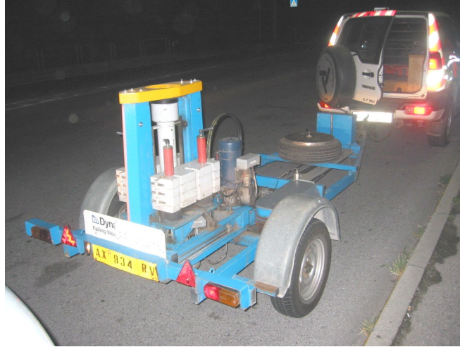
Figure 4: Bearing capacity survey on the main network of the Province of Milano
