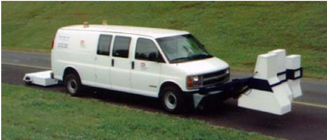
Figure 1: Pulse Radar GPR system developed under a small business innovative research program with the ERDC.
