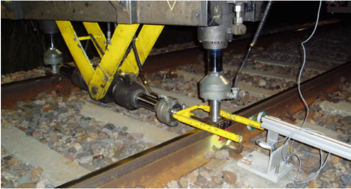
Figure 7: Arrangement of loading and measuring equipment at one of the test sleepers.
