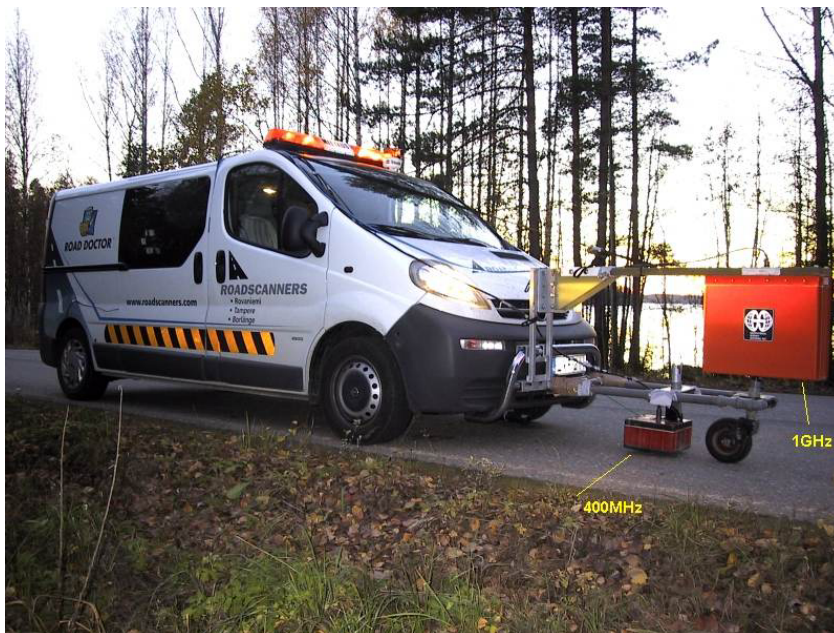
Figure 1 GPR survey car mounted with 1.0 GHz and 400 MHz antennas.
