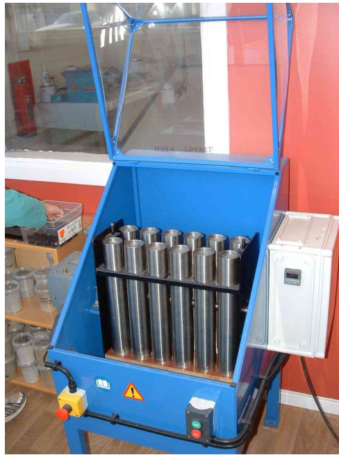
Figure 1: Mechanical shaker for the shaking abrasion test.
