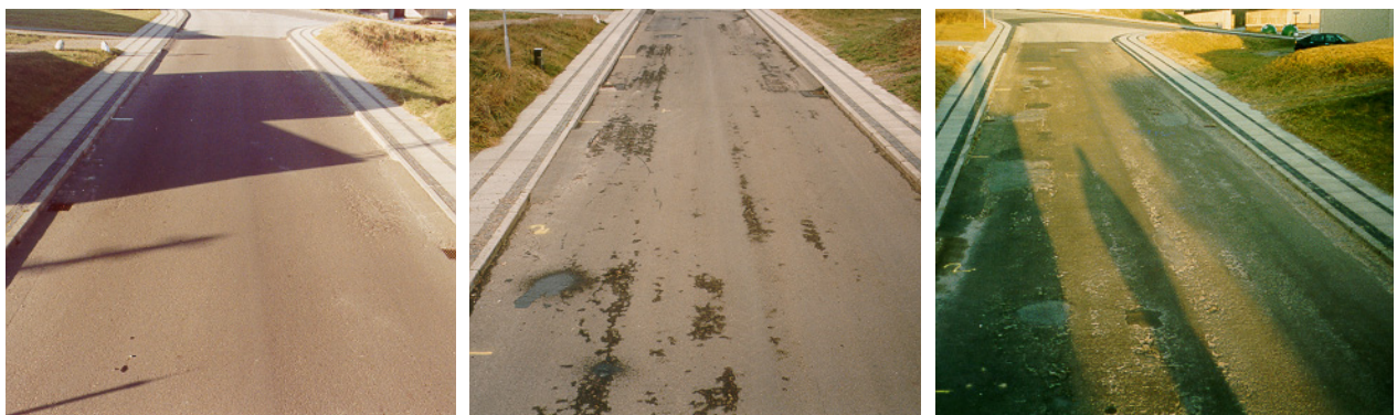
Figure 3. Example of visual condition of 10 metres of a test section in 1989, 1994 and 1999
