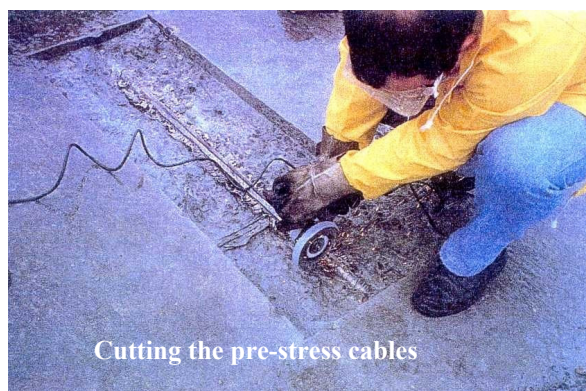
Figure 4: Assessment of in-situ pre-stresses in the concrete
