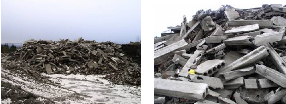
Figure 3: Element concrete stockpile
