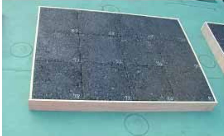
Figure 9: Specimens for atmospheric exposure tests
