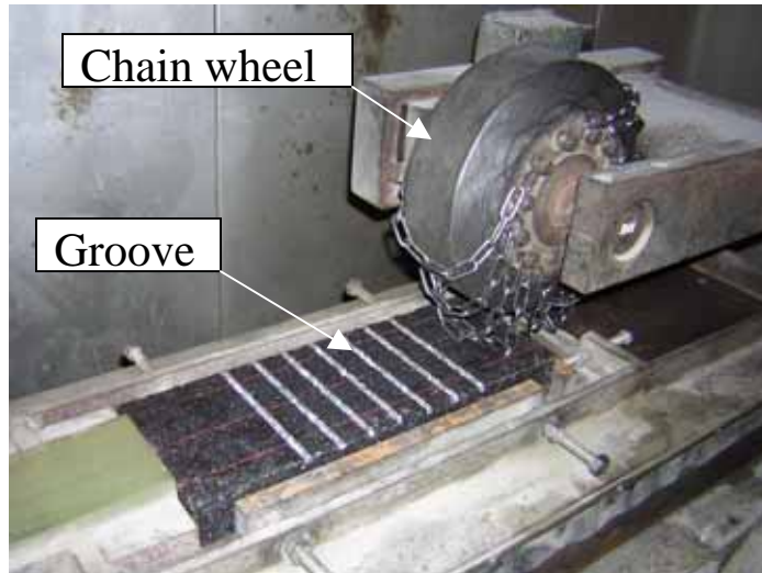
Figure 6: Specimen and a chain wheel for raveling test
