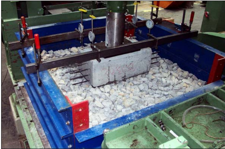
Figure 3: Ballast trough with USP
