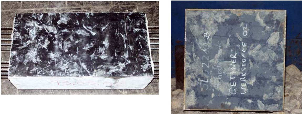
Figure 4: Surface of two USP after fatigue test with 8 million load cycles
