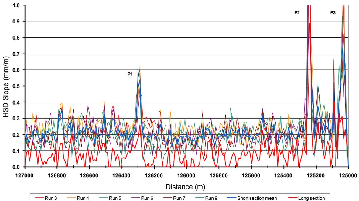
Figure 6: Comparison between HSD slope measurements on the motorway; short section runs and long section run.
