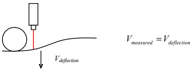
Figure 1: Velocity deflection measured with a Doppler sensor.
