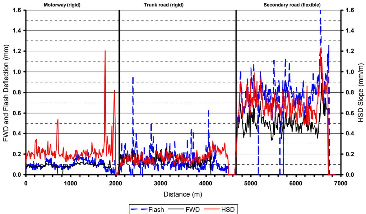
Figure 8: Comparison between HSD slope measurements, FWD and Flash deflection measurements on the three short sections.
