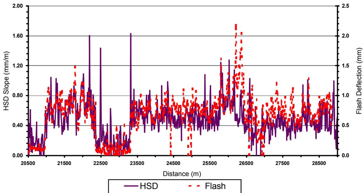
Figure 5: Comparison between HSD slope measurements and Flash deflection measurements on the flexible route.
