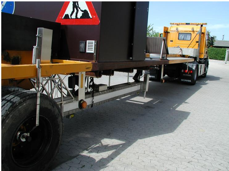
Figure 4: The towing truck, the semi trailer and the measuring sensors mounted on a stiff beam in front of the right hand side twin wheel. The stiff beam is servo controlled to keep the sensors focused.
