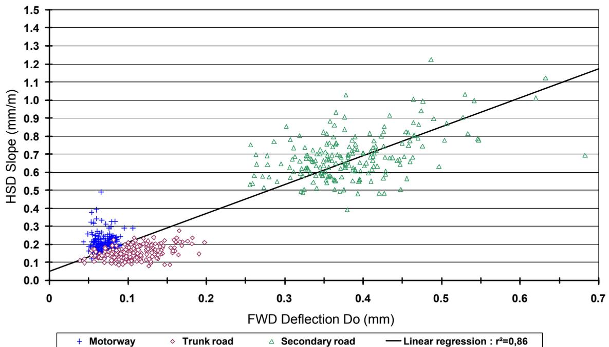
Figure 9: Comparison between HSD slope measurements and FWD deflection measurements  $D_0$ .
