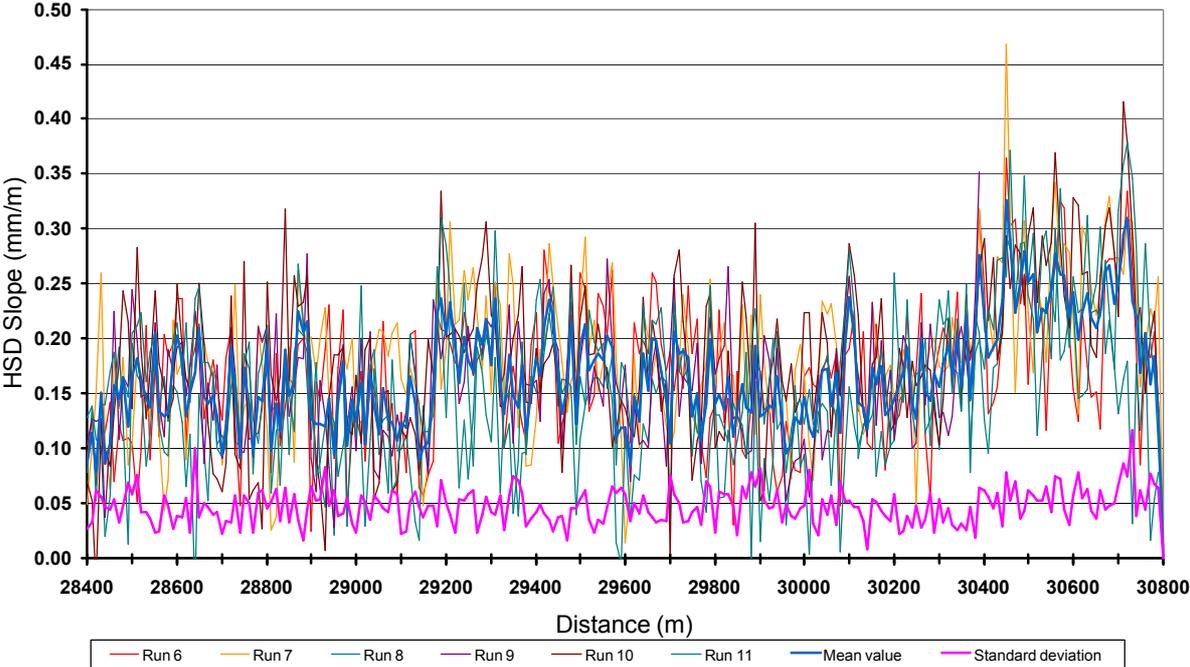
Figure 7: Comparison between HSD slope measurements on the trunk road short section ; individual runs, mean value and standard deviation.
