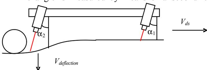
Figure 3: Principle of velocity measurement using 2 Doppler sensors.
