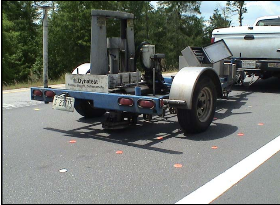
Figure 4: Dynatest FWD Model 9000 over instrumentation array.
