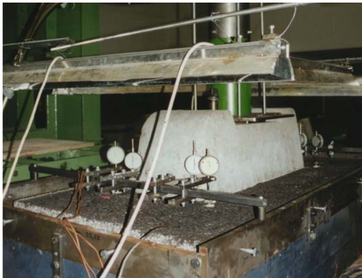
Figure 7: Test set-up to investigate erosion effects due to dynamic loading and frost-heave behaviour (unloaded condition).
