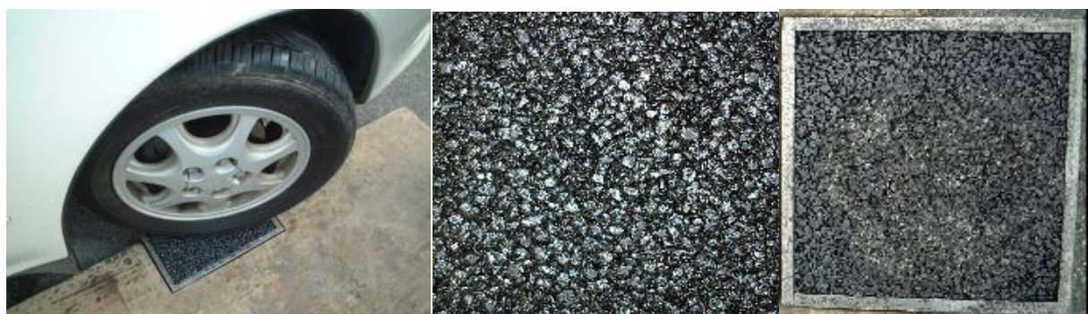
a) Alternating torsional load test by passenger car b) Sample surface condition before and after the test
