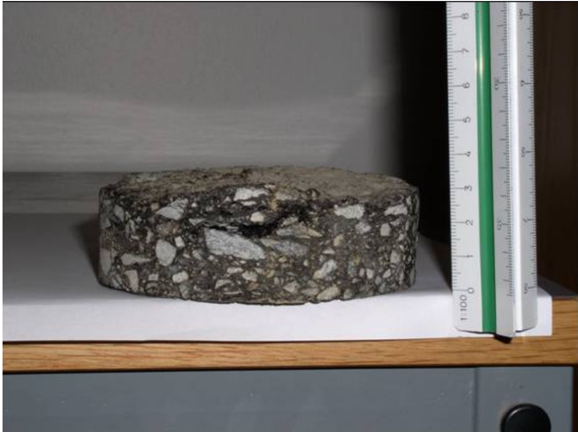
Figure 1: Thin and damaged sample (diameter 10 cm), unsuitable for further testing
