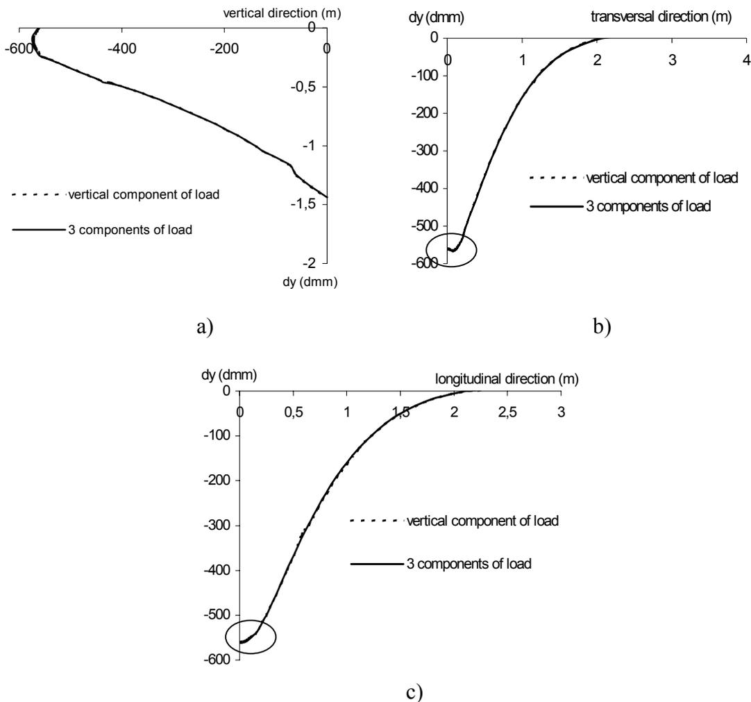
Figure 5: Superficial deflection with the vertical component and all components load:
