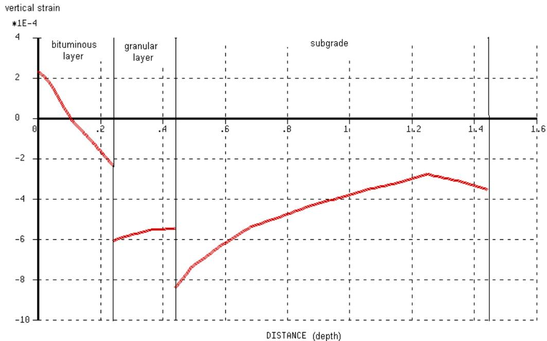
Figure 3: Evolution with depth of the vertical strain of structure 1 (all components of load).
