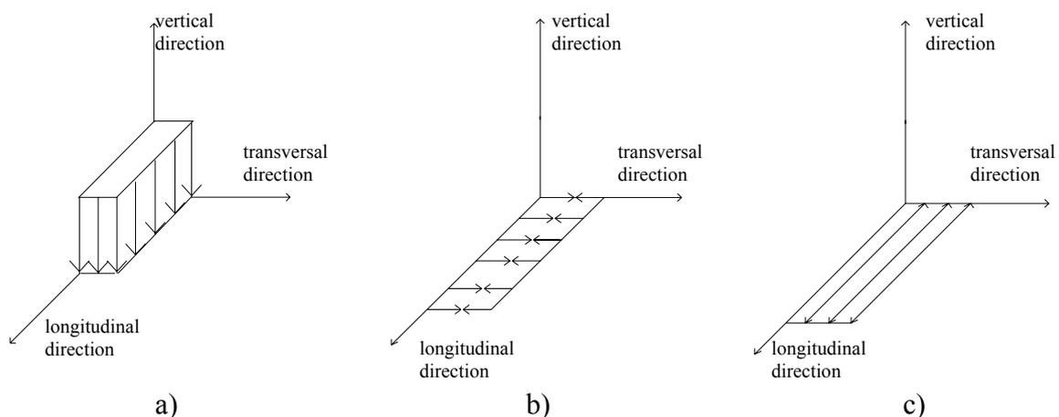
Figure 2: Contact stress directions: a) vertical; b) transversal; c) longitudinal.
