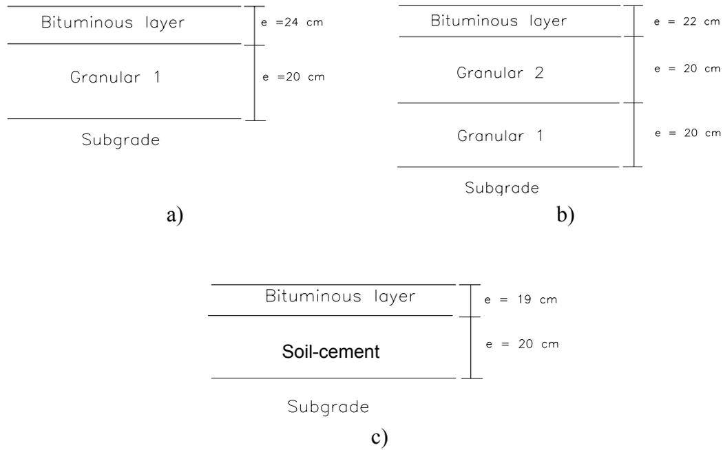
Figure 1: Geometry of the pavement sections considered in the numerical study: a) structure 1; b) structure 2; c) structure 3.
