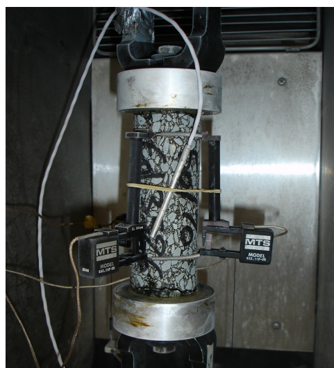
Figure 2: Mix sample to be tested on the hydraulic press.
