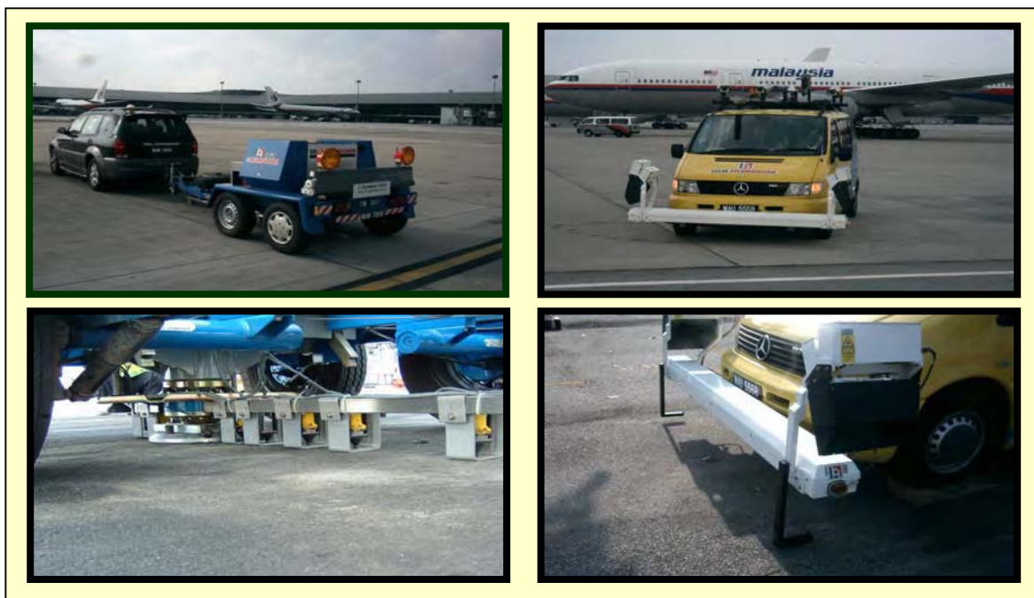
Figure 4: Bearing Capacity Data collection using the HWD and Multi Laser Profilometer
