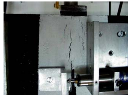
HaTelit ® C- reinforced sample after 490.000 cycles
